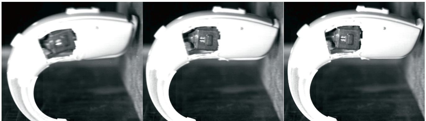
Image 4. High-speed video is used to record impact. Left photo is 0.9 after impact, middle is 0.1 after impact, right is at impact. Note motion of receiver at center of device.
