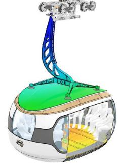
The linear and nonlinear structural performance of CATIA designs – from parts to assemblies – can be evaluated quickly using Abaqus-based structural simulation applications on the **3D**EXPERIENCE platform.
