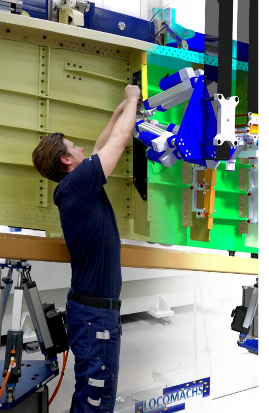
A research and development project called LOCOMACHS (Low-Cost Manufacturing and Assembly of Composite and Hybrid Structures) is a perfect example of this. Comprising 31 key European players in the aircraft industry, LOCOMACHS develops technologies that produce and assemble composite parts faster by mitigating time-consuming operations that generate recurring costs for production lines.
